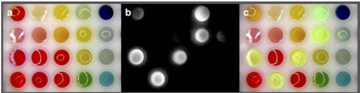
Fig. 7 NIR laser light delivered through hand-held laser wand for demonstration of NIR laser beam guidance by augmented microscope. (a) Visible image conceals location of NIR laser beam, (b) NIR image lacks any spatial information, (c) augmented image visualizes both NIR light and visible spatial cues.
